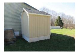
This 4.5-ton outside residential bulk wood pellet storage bin has a ventilated soffit and two ports for pellet delivery
