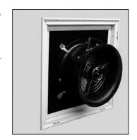
**Note:** The Duct Blaster fan can also be attached to the filter slot using cardboard and tape.
